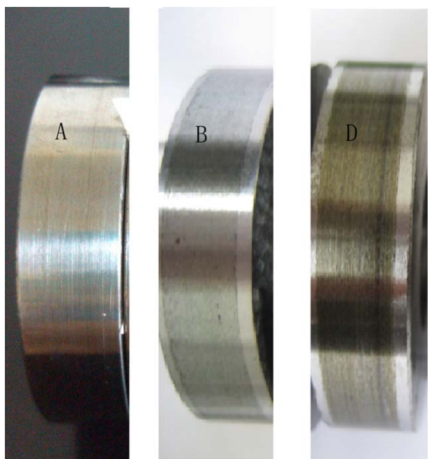
Figure 8. Transfer film on the steel ring. [Color figure can be viewed in the online issue, which is available at wileyonlinelibrary.com .]
